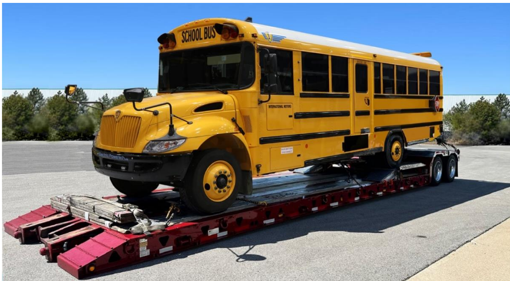
Figure 29. Towing on Flatbed / Lowboy Trailer
