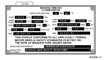
Typical Axle, Tire, and Rim Specifications-Vehicle Identification Label
