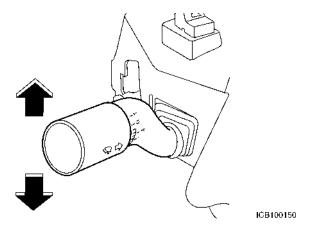
Move the turn signal lever up or down to the full turn position which is past the point of resistance. The turn signal automatically cancels if the steering wheel is turned through a large enough degree.
