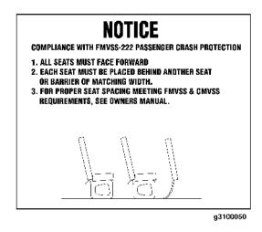
The standard track seat label is found on the front bulkhead of all buses with track seating.
