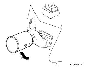
Pull the turn signal lever past the click position, the lights switch to high-beam position. Pull again to return to low-beam.
