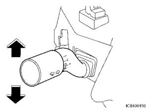
Some switches include a lane change feature, which allows you to signal your intention to change lanes without locking the switch into the full turn position. Move the turn signal lever, up or down, to the point where resistance to movement is felt. The turn signal lever returns to the OFF position when released.
