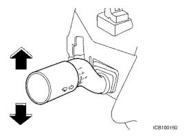
The turn signal switch is located on the left-side of the steering column and is part of the multifunction switch. Move the lever up or down to signal the turning direction. After the turn has been completed, the turn signal automatically cancels.
