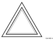
Use the triangle whenever the bus is pulled over to the side of the road. The reflective triangle kit is usually located behind the driver's seat. After opening the kit, unfold the triangle and make sure it locks in place.
