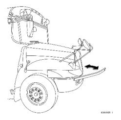
The crossing gate extends when the RED warning lights are on to make sure that students do not cross too close to the front of the bus and out of the view of the driver.
