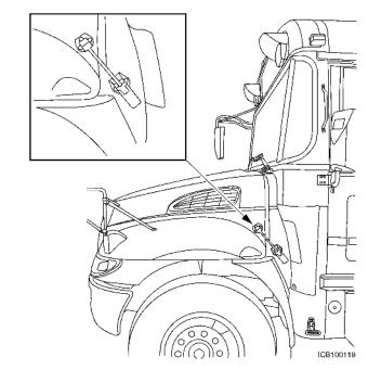
Release the latches on both sides of the cowl.
