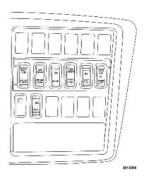
CRUISE SWITCH: Turns the cruise control system ON and OFF.
