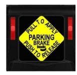
This is now the equivalent of the parking brake knob popping out at 30 PSI or the spring brake applying itself automatically at 30 PSI.
